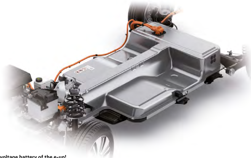
The high-voltage battery of the e-up!
