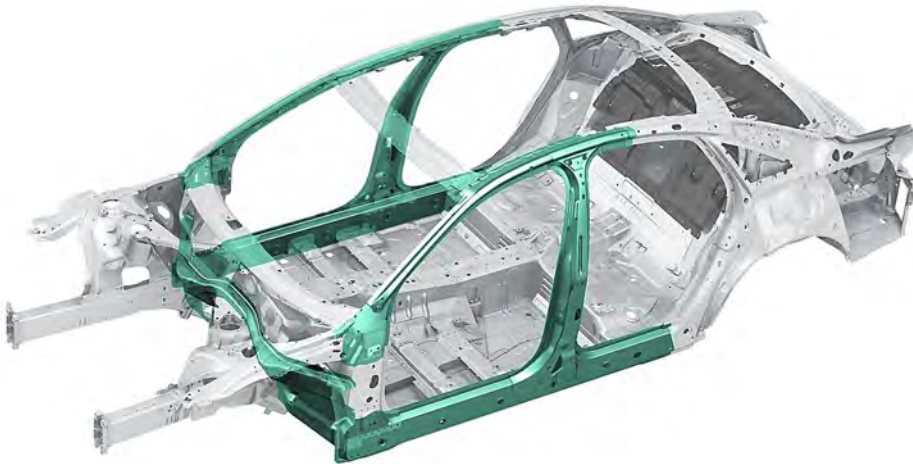
Body with reinforced passenger compartment
