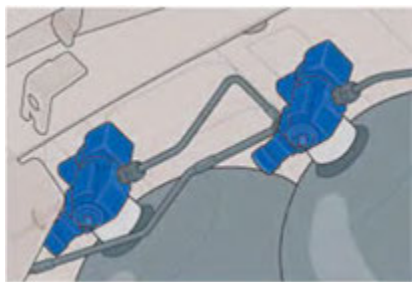
Electromagnetic shut-off valves on the gas tanks
