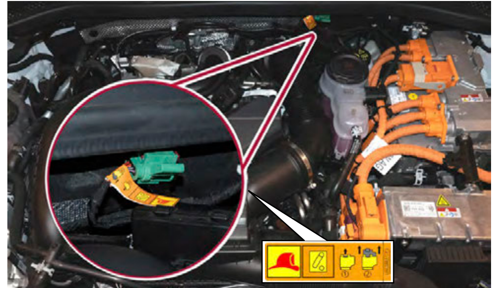
Cut-out connection in the engine compartment of hybrid vehicles. See also " Previous identification ".
