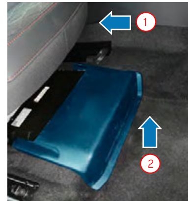
Disconnecting the 48-volt vehicle electrical system in mild hybrid vehicles (MHEV).
