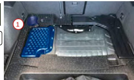
Example for disconnecting the 12 V system in a Leon PHEV.
