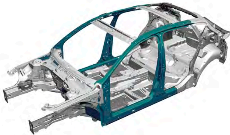
Body with reinforced passenger compartment
