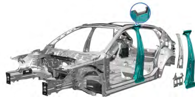
B-pillar with multi-shell structure
