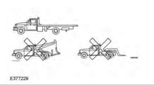
Do not tow a vehicle that has been involved in an accident on its drive axles.
