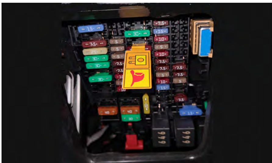
Cut-out connection in the passenger compartment, dash panel on the fuse carrier.
