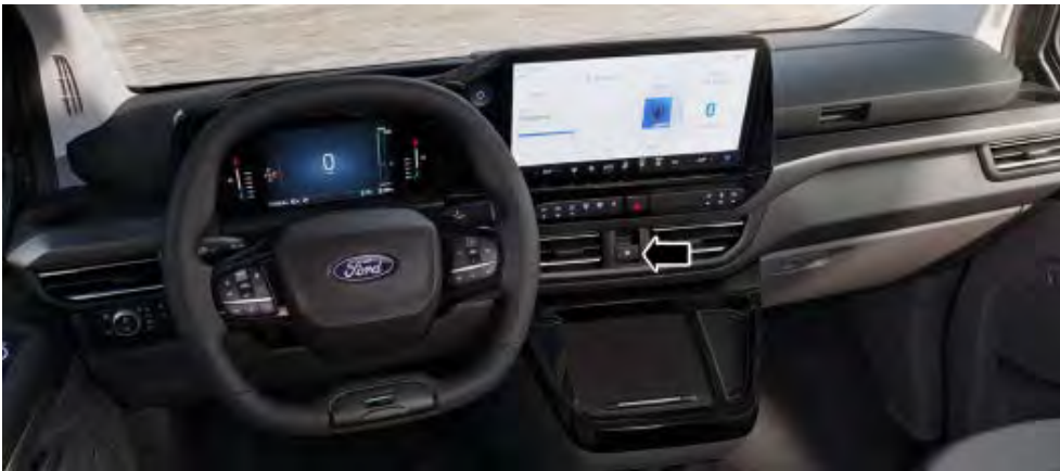
Conventional vehicle with automatic gearbox: apply electronic parking brake or pull handbrake lever.
