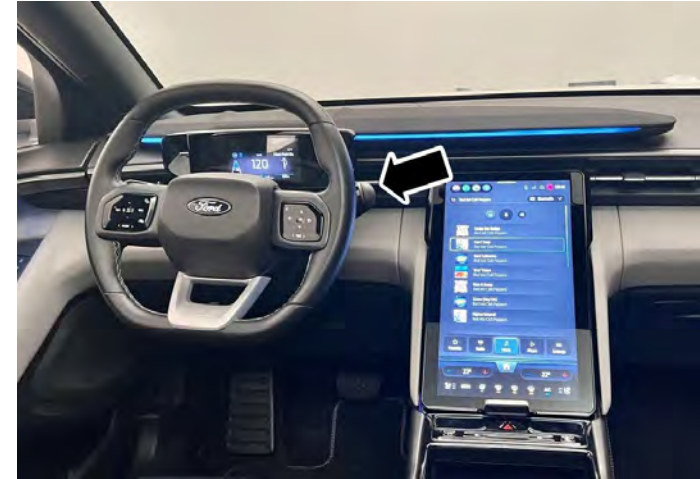
Operate the electronic parking brake on the right-hand steering column switch.
