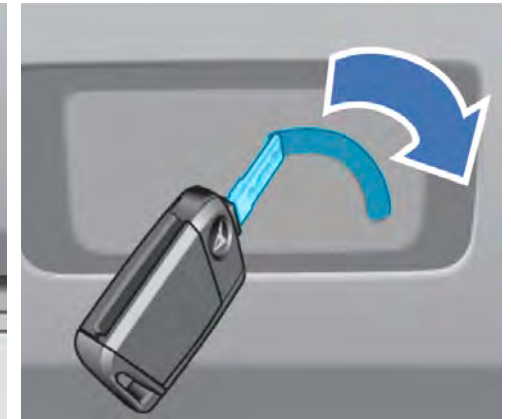
Enter the key in the slot and slide it to unlock
