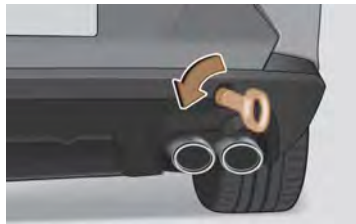
Fastening of the rear towing eye
