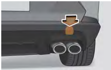
Access cover to the rear towing eye
