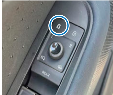
Deactivate the childproof lock electronically in the door trim.
