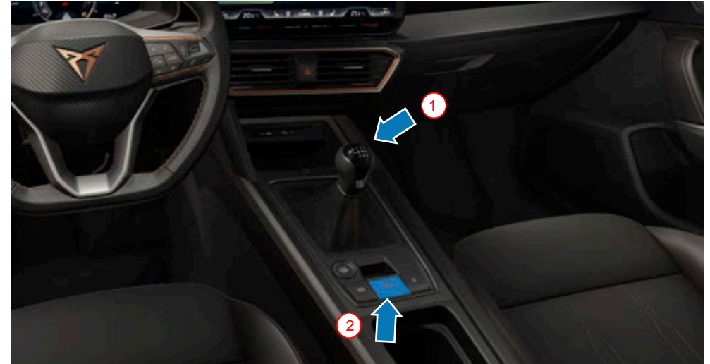
Vehicles with manual gearbox: place the gear lever (1) in the “Neutral” and activate the electric handbrake (2).
