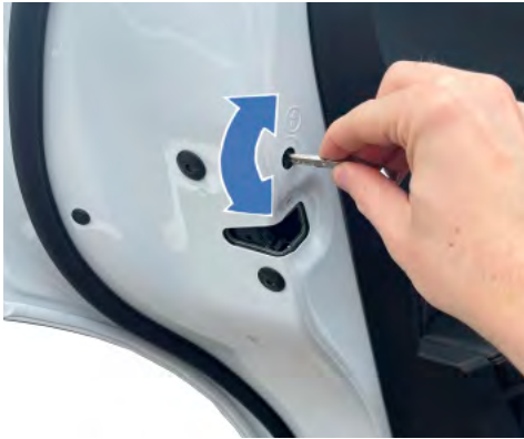
Deactivate the childproof lock mechanically using the key.
