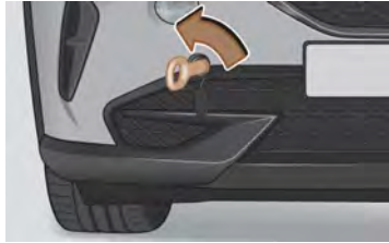
Fastening of the front towing eye
