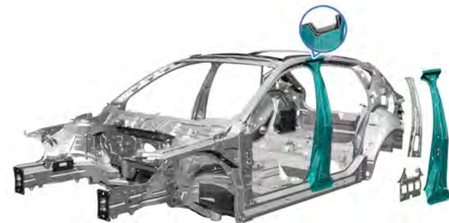
B-pillar with multi-shell structure
