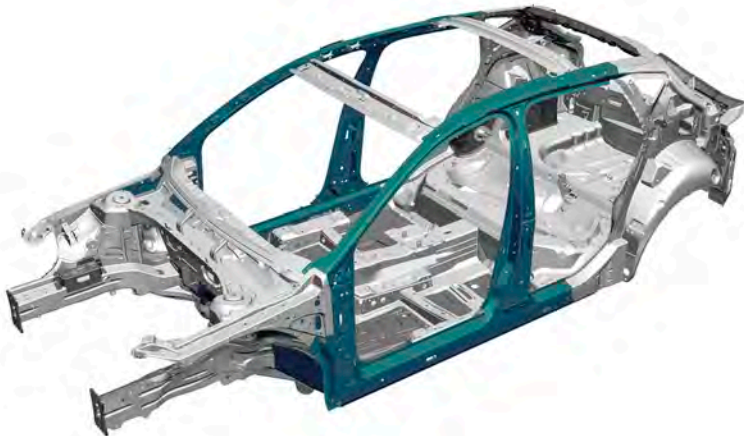
Body with reinforced passenger compartment
