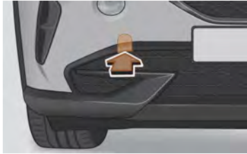
Access cover to the front towing eye
