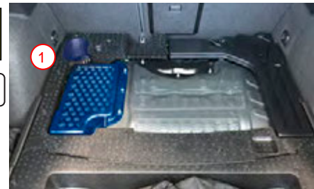
Example for disconnecting the 12 V system in a León PHEV.
