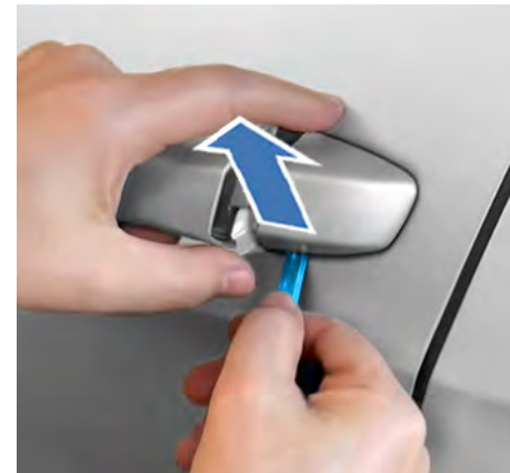
Remove the lid by levering with the key
