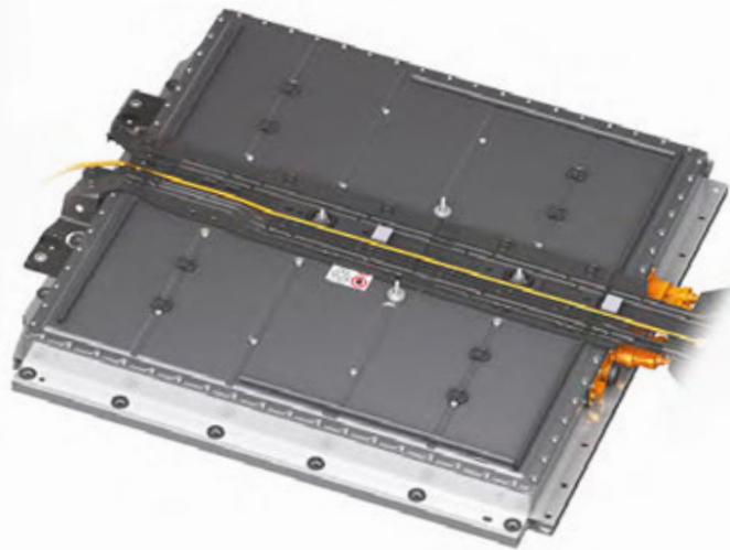
The high voltage battery of the BORN
