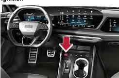
Press the "Start-Engine-Stop" button in the centre console without operating the foot brake.
