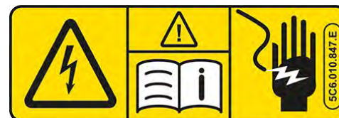
Examples of warning stickers in high-voltage vehicles:
